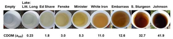
**Above:** smartphone photos of a 2-gallon white bucket filled with lake waters with increasing  $a_{440}$  left to right.
