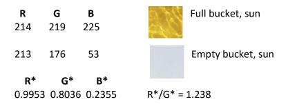
Using the above best-fit equation the calculated CDOM is:  $a_{440} = 3.6 \text{ m}^{-1}$  versus a measured value of:  $a_{440} = 4.5 \text{ m}^{-1}$ .
